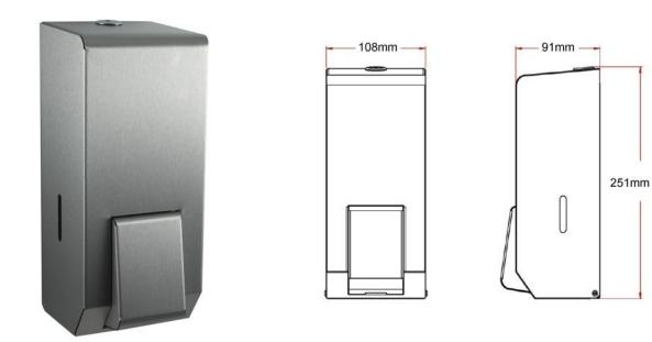
Model WAPL20 is our wall mounted sanitizer or liquid soap dispenser. The soap and sanitizer dispenser is manufactured from grade 304 stainless steel polished to a satin finish. Supplied with concealed fixings and has a capacity of 0.9 litres of hand sanitizer or liquid soap. The soap / sanitizer reservoir is provided with a hinged lockable front to aid refilling and to resist vandalism.
